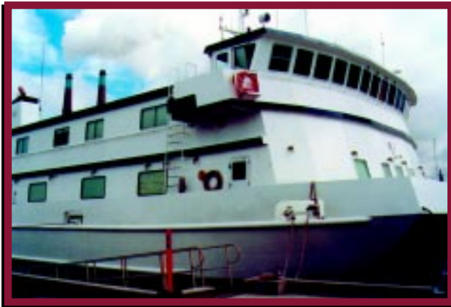
America's premier deep-sea research vessel is 36 meters long. It's primary mission is to provide a stable platform for deploying, operating and recovering a tethered, remotely operated, deep sea vehicle which can dive to a depth of two miles.
